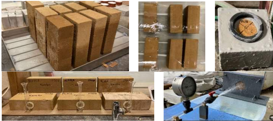
Figure 1 – Water resistance characterization of CSEB: capillary water absorption (left top); water absorption by immersion (center top); water permeability (right top); low-pressure water absorption (left bottom); spray test – accelerated water erosion (right bottom)
