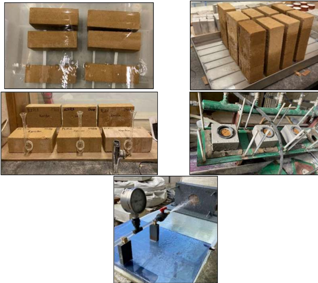
Figure 1 – Blocks characterization: a) absorption by immersion; b) absorption by capillarity; c) low-pressure water absorption; d) water permeability; e) spray test
