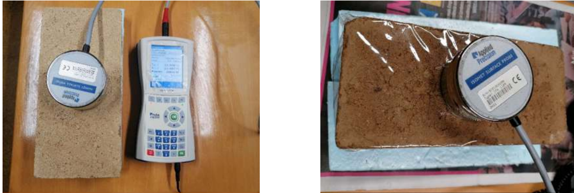
Figure 40 – Thermal conductivity test: a) ISOMET 2114; b) surface probe over plastic wrapped saturated surface dried CEB
