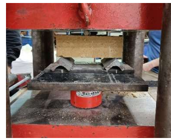
Figure 15 – Bending tensile strength test
