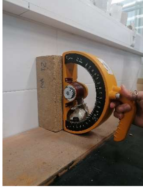
Figure 29 – Pendular sclerometer test
