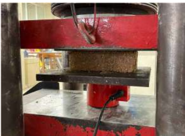
Figure 13 – Compressive strength test
