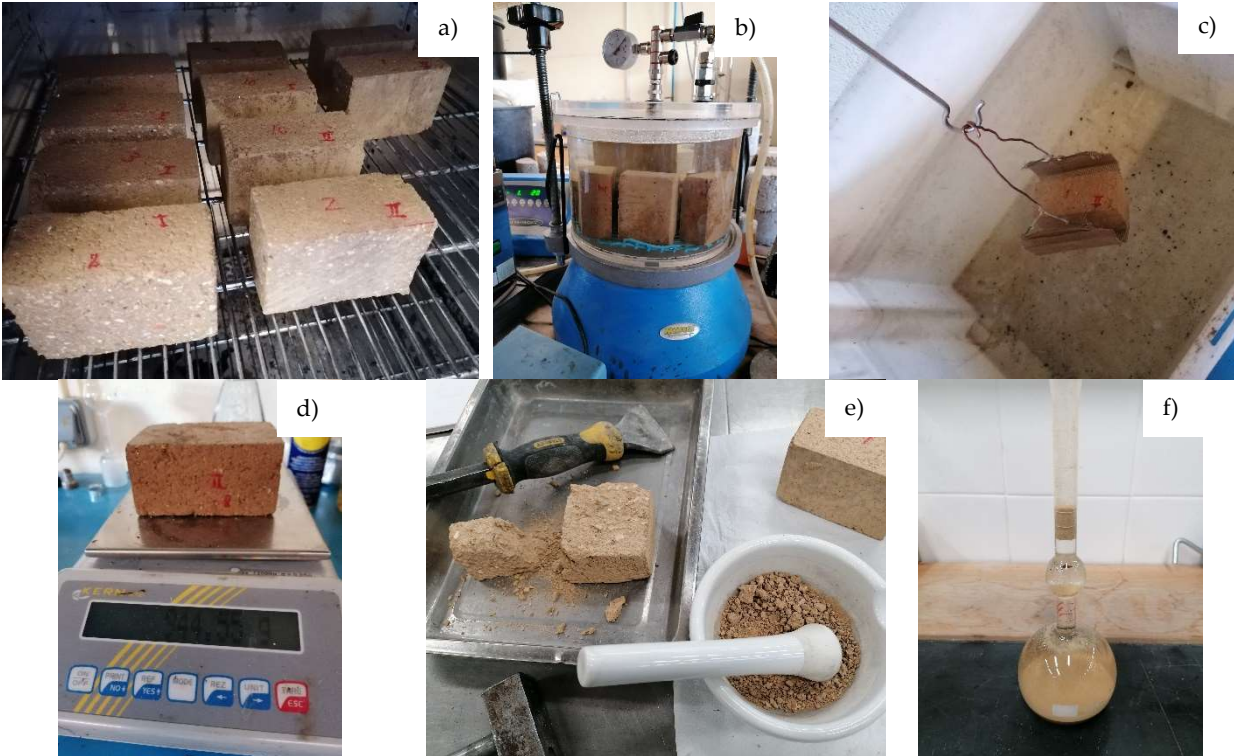
Figure 1 – Total porosity test: a) oven-drying; b) saturation; c) immersed weighing; d) saturated surface dry weighing; e) particle size reduction; f) particle density
