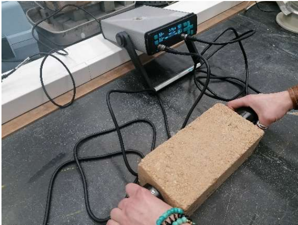
Figure 8 – Ultrasonic pulse velocity test
