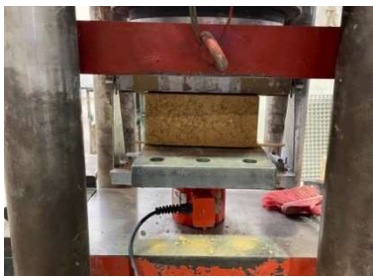
Figure 14 – Splitting tensile strength test
