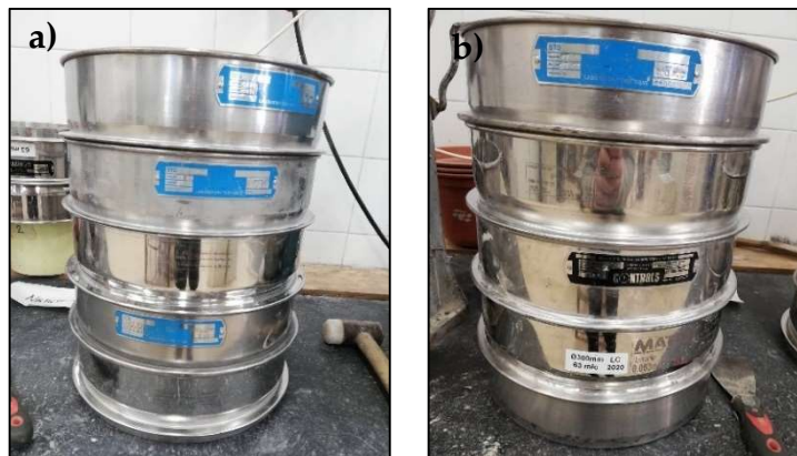
Figure 2 - Sieve column: a) No. 2.5, No.3.5, No. 5, No. 10 and No. 18; b) No. 35, No. 60, No. 120 and No. 230
