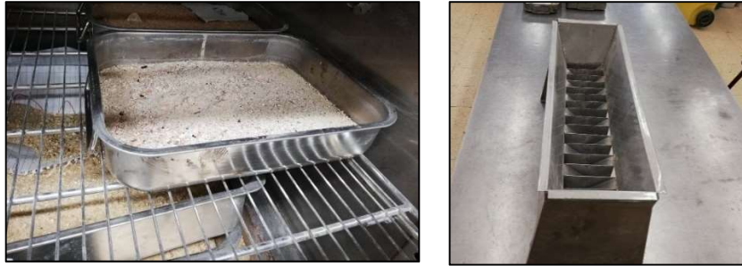
Figure 1 - Drying of the sample in a ventilated oven and reduction of it by quartering
