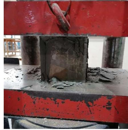
Figure 7 – Compressive strength test setup
