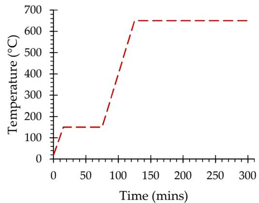
Figure 15 – Thermal treatment procedure
