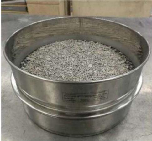
Figure 12 – Sieving of source concrete particles
