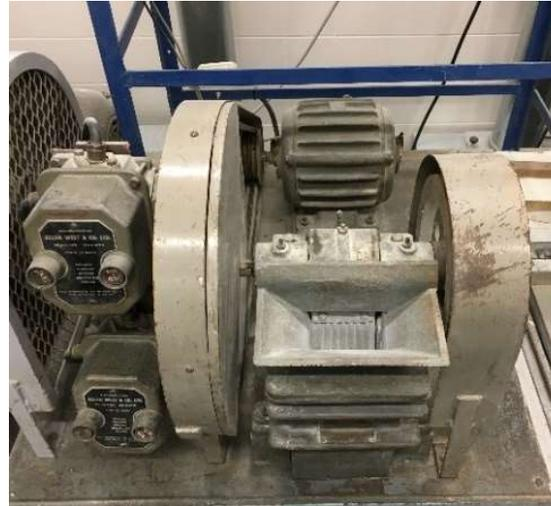
Figure 9 – Jaw crusher with a jaw opening of 1cm
