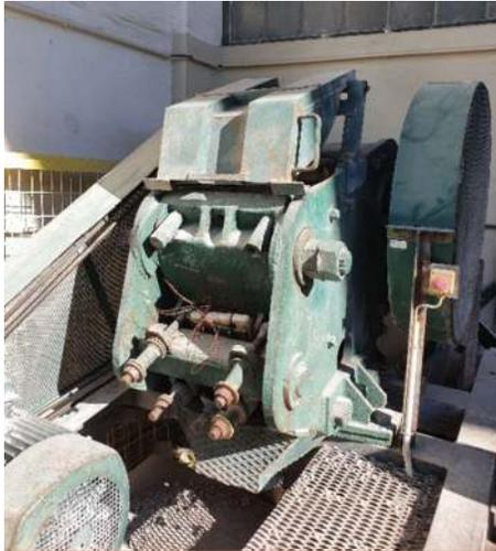
Figure 8 – Jaw crusher with a jaw opening of 2cm
