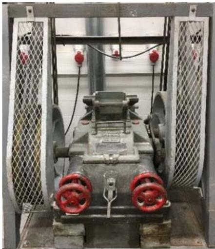
Figure 10 – Roller mill
