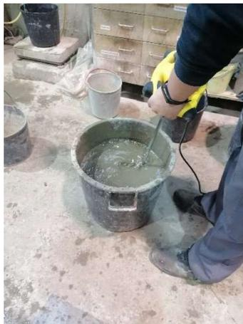
Figure 1 – Source cement paste production
