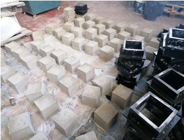
Figure 3 - Source cement paste cubes
