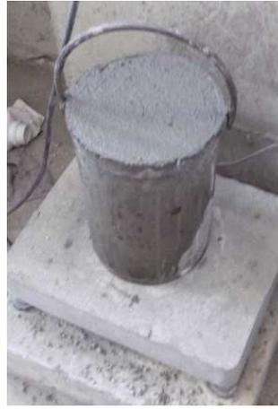
Figure 6 – Fresh density test setup
