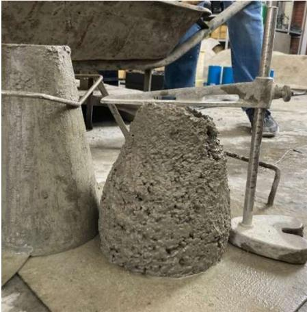
Figure 5 – Slump test setup
