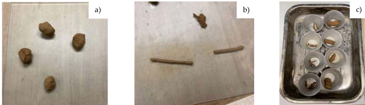
Figure 8 – Plasticity limit test: a) soil preparation; b) cylindrical filaments with a diameter of 3 mm; c) placement of the samples in capsules
