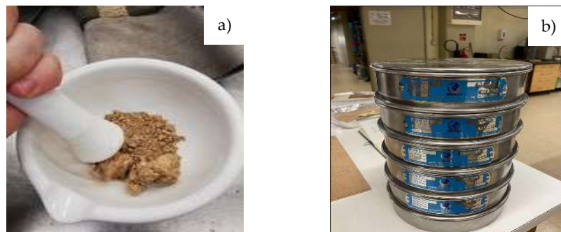
Figure 1 – Particle size distribution: a) breaking of soil sample clods; b) sieve series
