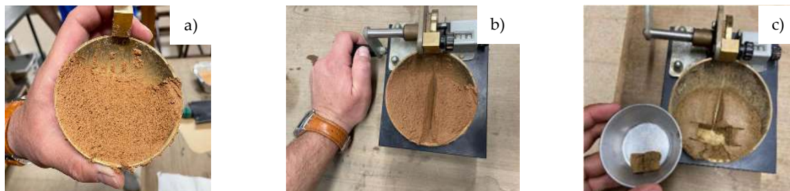
Figure 6 – Liquidity limit determination: a) mixture of soil and water and placement on the Casagrande shell; b) 2 mm wide groove; c) collection of the sample
