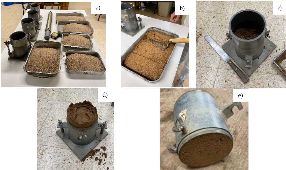
Figure 13 – Compaction test: a) division of the soil into 2.5 kg portions; b) preparation of each portion; c) introduction of the soil in the cylindrical mould; d) excess soil in the mould; e) mould ready for weighing
